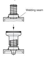
To prevent damage of the plastic knob, it will be driven onto the shaft using a plastic mallet, after the welding process.
